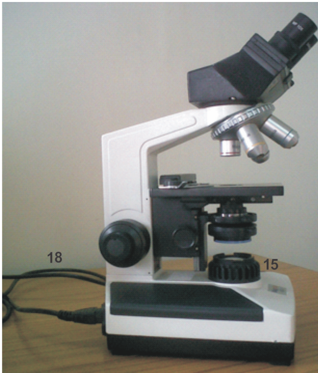
Fig. 5.19: A binocular compound microscope in side view showing light source (15), and an electricity input cable (18).
