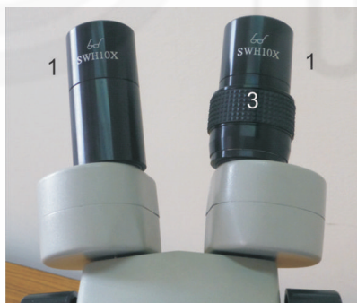
Fig. 5.4: A portion of the head of stereo microscope in front view showing two eyepieces (1). The eyepiece on the right hand side has a ring-like structure – the diopter (3).
