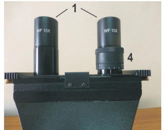
Fig. 5.13: A portion of head of binocular compound microscope in front view showing two ocular lenses. The ocular on right hand side has a ring-like structure known as the diopter.
