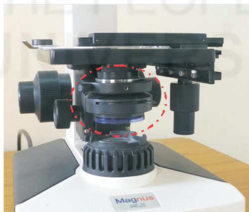
Fig. 5.18: A binocular compound microscope in an angular, front view showing condenser lens assembly unit in a lowered position.
