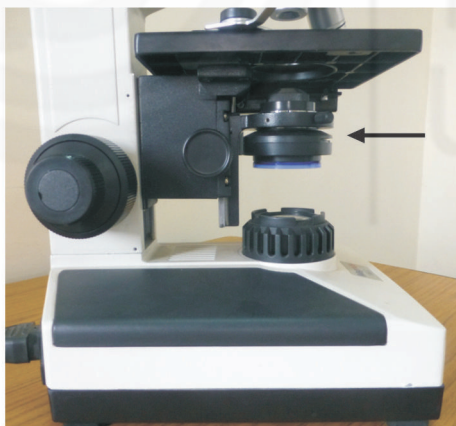
Fig. 5.17: A binocular compound microscope in side view showing condenser lens assembly (arrow) near the stage.
