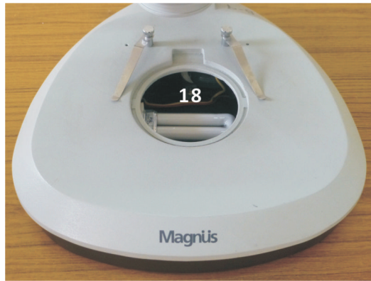
Fig. 5.8: Base of the stereo microscope in front view showing stage light (18).
