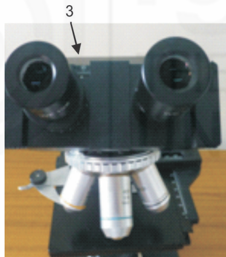
Fig. 5.14: A portion of head of binocular compound microscope in front view showing an ocular slide in a closed position (left-hand) and in opened position (right hand).
