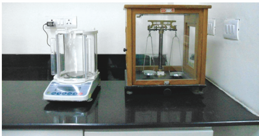
Fig. 3.5: A dry bench with coarse and fine balances.
