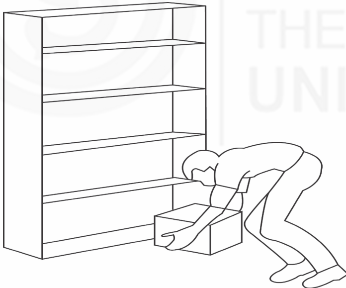
Fig. 3.11: Heavy objects should be placed at a convenient height to avoid back strains.
