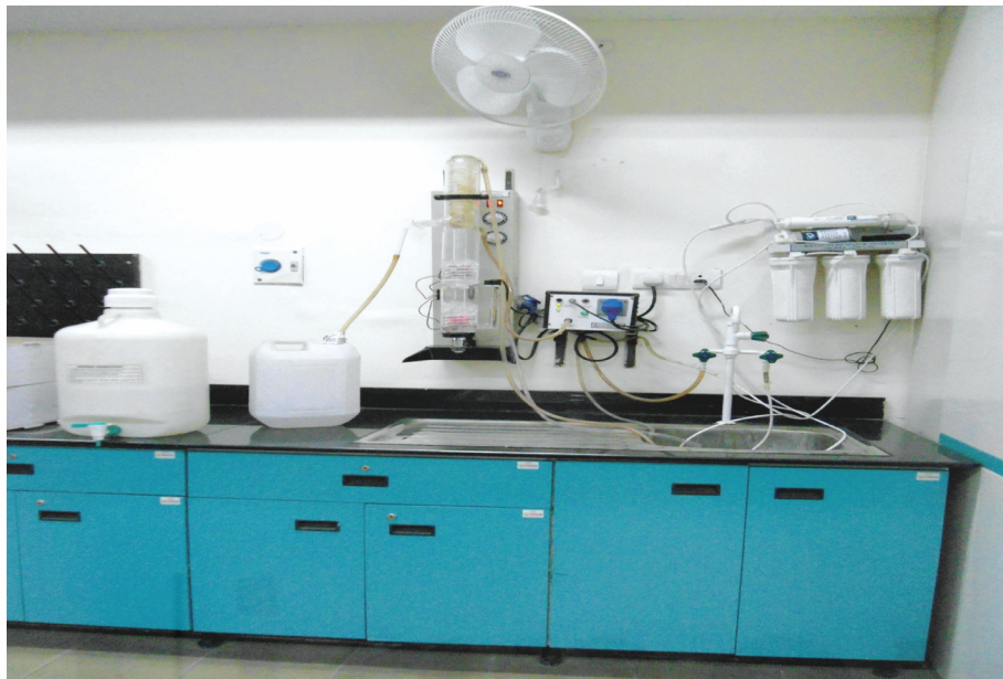
Fig. 3.4: A wet bench with a distillation plant.
