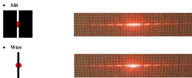
Fig. 9.3: Intensity distribution in the diffraction patterns of a single slit and a wire.
